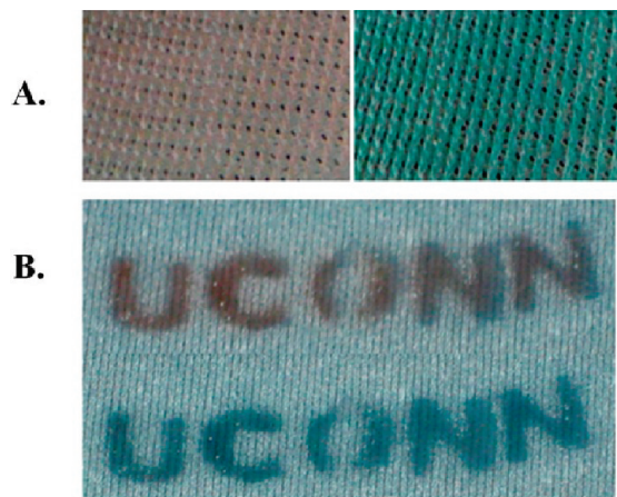
Figure 15. Demonstration of electrochromism on fabric electrodes with a soluble EC polymer spray-cast onto a Spandex fabric electrode. (A) EC polymer-coated Spandex in electrolyte bath, stretched, switching between neutral (left) and oxidized (right) states. (B) Patterned EC polymer on fabric electrode in neutral (top) and oxidized (bottom) states. Adapted with permission from ref 87. Copyright 2010 American Chemical Society.
