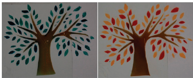
Figure 14. Pattern obtained by spray-casting through a shadow-mask of a variety of available EC polymers as discussed in the previous sections. Reproduced with permission from ref 34. Copyright 2010 American Chemical Society.
