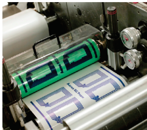
Figure 16. Use of flexoprinting to print PEDOT:PSS layers on flexible substrates at Acreo. Reprinted with permission from Acreo AB. 76
